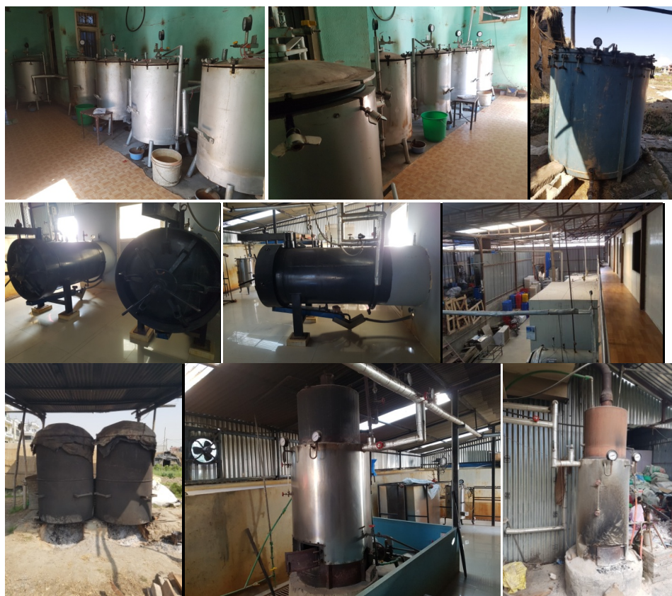
Fig. 7. Big-sized autoclaves with capacity ranging from 200 l to several thousand liters, using firewood as fuel source.
