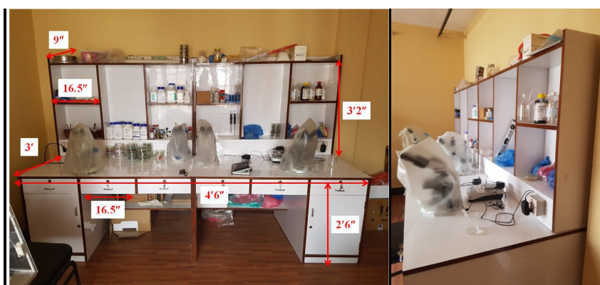
Fig. 3. Size of one-sided working table. Left, front view and right, side view.
