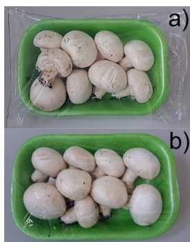
Fig. 11. Button mushrooms packaged in the bionanocomposite-based laminate/EPS tray (a) and in the conventional PVC stretchable/EPS tray configuration (b) (Gholami et. al. 2017).
