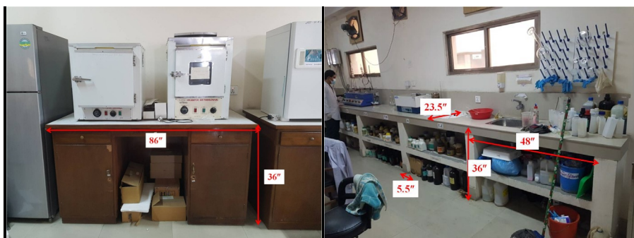
Fig. 5. Size of table with drawers and cabinets (left) and slab with wash basin sink and storing space.
