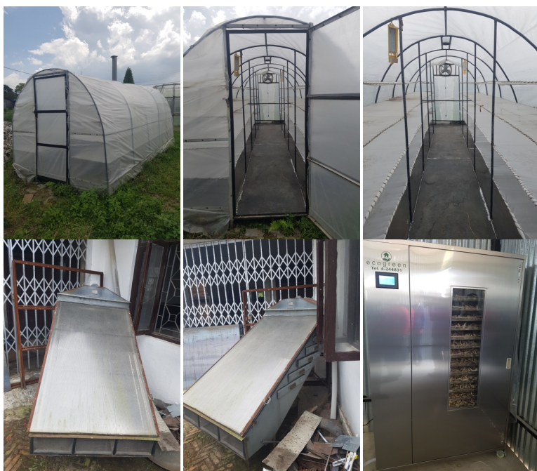
Fig. 13. Solar dryers (plastic house and cabinet model) and electric dryer.
