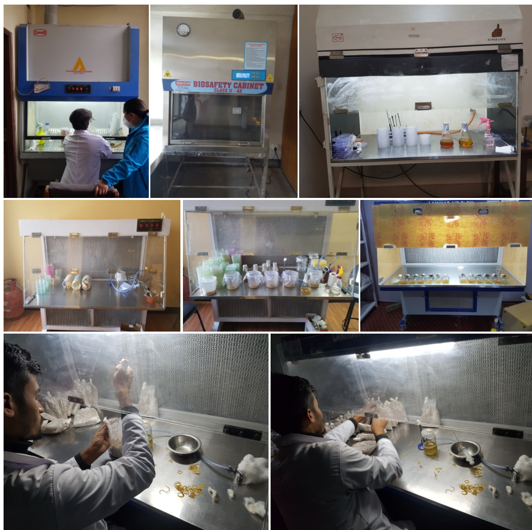
Fig. 8. Biosafety cabinet and laminar air flow cabinet for inoculation purposes.
