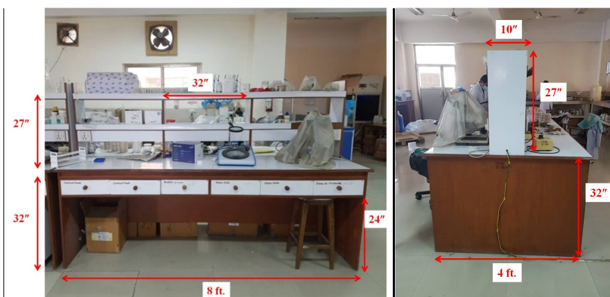
Fig. 4. Size of both-sided working table. Left, front view and right, side view.
