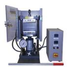
(Model Mini CH) Twelve ton manual, two-column hydraulic lab press with digital heated platens. Easy-to-read dual scale analog gauge, reading in pounds force and metric tons. Electrically heated platens for temperatures up to 650 deg F (343 C upon request) with digital controller per platen. (picture shown with analog gauge)
